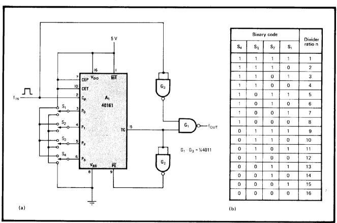
**Binary breakup.** Single counter and three gates simplify design of variable-modulo divider (a). Binary switches  $S_1 - S_4$  set counter to 16 - n, where n is desired divider ratio (b). Output of gate  $G_1$  is a pulse with a frequency equal to  $f_{out} = f_{in} / n$ , for  $1 \le n \le 16$ .
